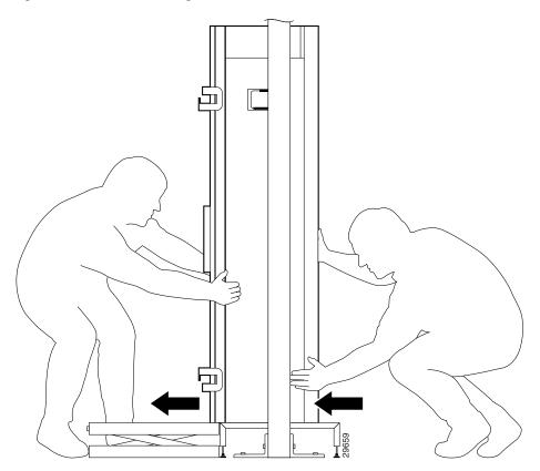
Step 5 With one person positioned on the side of the router to prevent it from tipping, install the four chassis anchor clips through the slots in the bottom of the chassis, align the holes with the bolt holes in the platform, and insert and tighten the four bolts to prevent the chassis from shifting on the scissor-jack platform. (See Figure A-5.)
